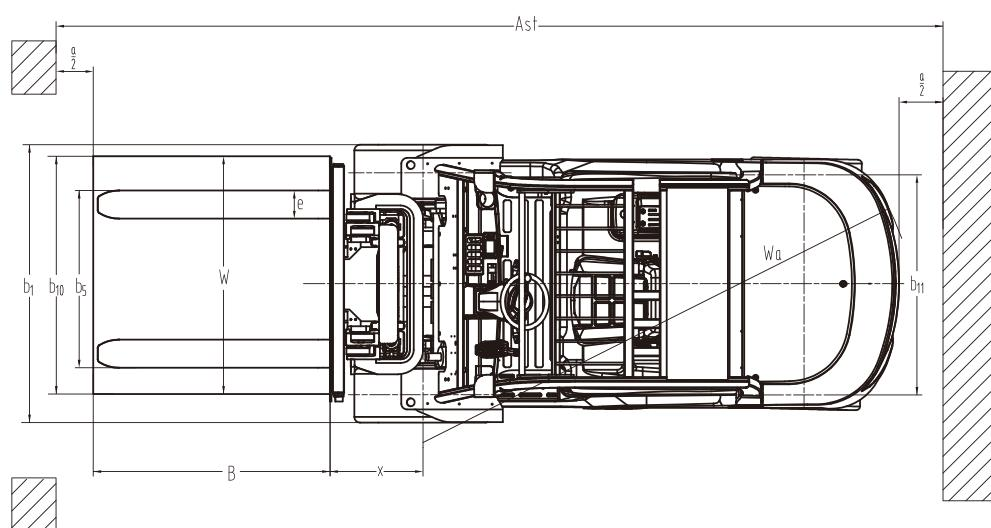
$A_{st} = B + X + W_a + \alpha$       B: Length of load or forks which is longer       $\alpha = 200\text{mm}$  safety clearance
