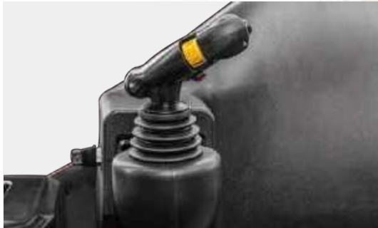
The multifunction control handle's unique shape and angle design helps minimize hand movements and muscle fatigue.
