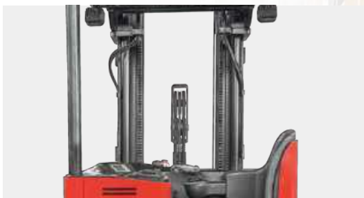
The optimized design of the wide-view mast enables the operator to get a better view, and improves the operation safety.
