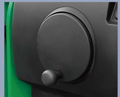
The LORD steering gear with torque feedback is provided to enable higher operating safety and operator comfort.
