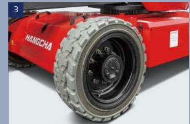
Tires: foam-filled tires with good off-road performance
